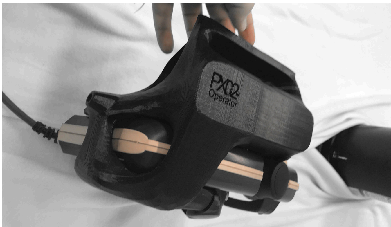
Figure 5. PX-Alpha Operator--Iteration PX02, 3D-printed prototype connected to KUKA KRC4 teach pendant controller (Image by the Author).
