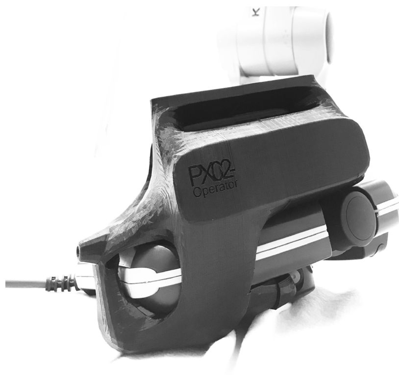
Figure 4. PX-Alpha Operator--Iteration PX02, 3D-printed prototype connected to KUKA KRC4 teach pendant controller (Image by the Author).
